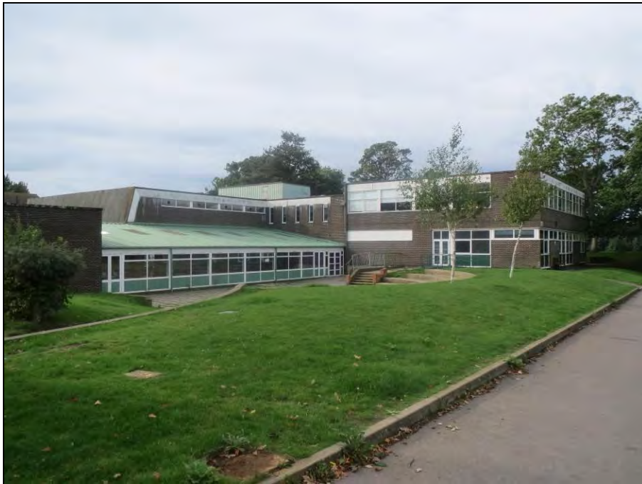
Plate 2.17 Western end of the northern elevation, situated to the south of a semi-circular low-level forecourt. The ground level section is constructed using prefabricated steel framed panelling, with large external windows and glass panelled doors, facing west (6959-0042)
