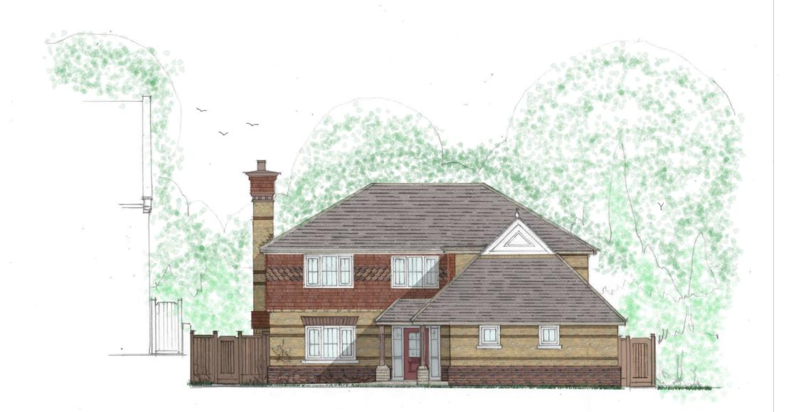
Revision-A- Roof pitch reduced to 30 degrees to lower ridge level. SRC 14.12.2017 B - Accomodation over garage reduced and roof shape and size revised. SRC 25.04.2018
